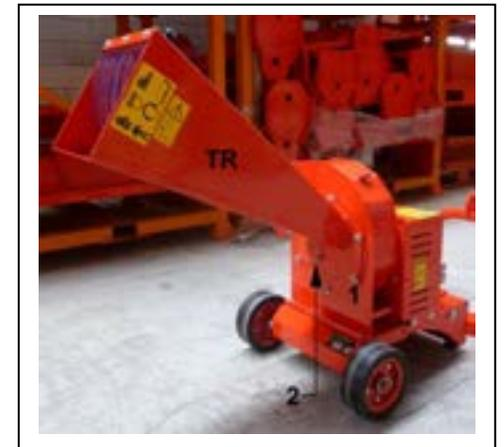
1. Take out from the carton box the machine “MAT”, the hopper “TR”, the III° point bracket “SU”, the III° point “TI”, the safety plastic cover “CU” and Use and maintenance manual of machine.
